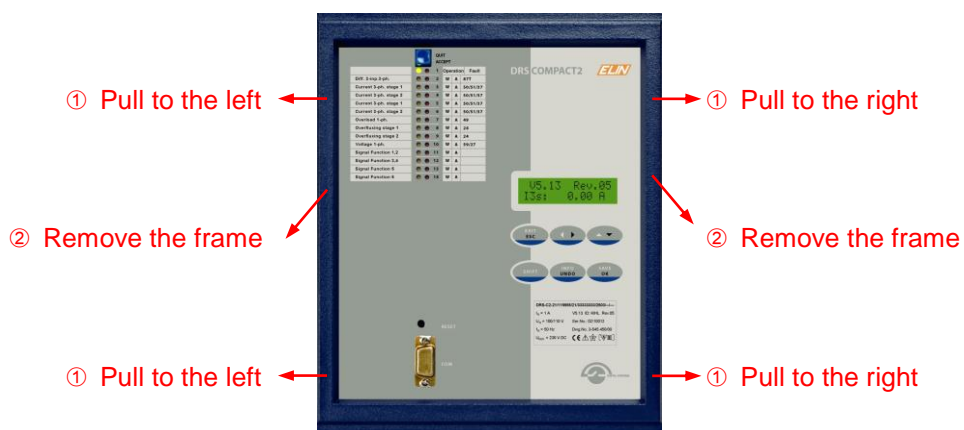
Fig. 20 Access to the UAKB module
