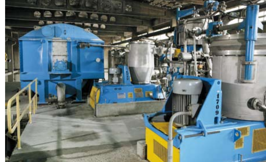
The new Andritz stock preparation system delivers high-quality pulp for the top layer without the addition of expensive kraft pulp.
