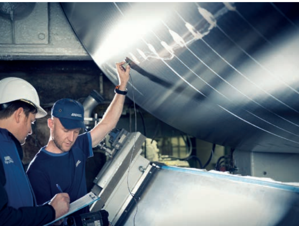
◀ On-site machine check of Yankee shell thickness.
