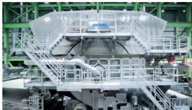
◀ St. Croix specified a large Steel Yankee (18-foot diameter) for both machines. TM1 started up in March and TM2 in July 2016.
