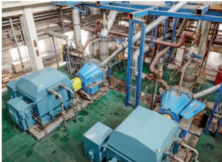
▲ High-consistency refiners in the newest P-RC APMP line at Sun Paper, Yanzhou
