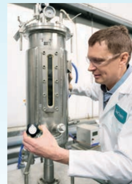
▲ Brian O'Neill with the "Seed Tank 0" vessel where the first 2 ml of Moorella is placed to start the fermentation process.
