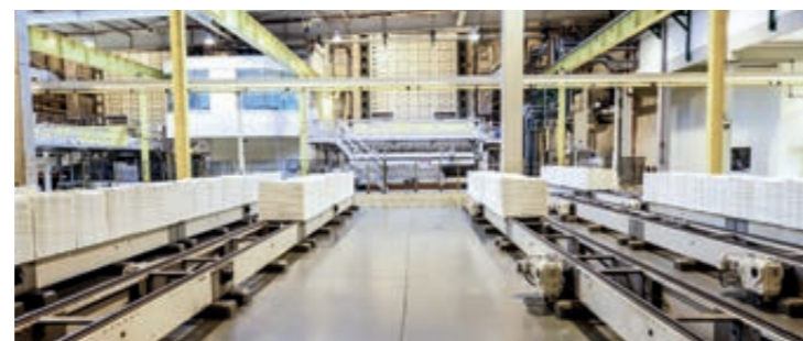
◀ One of the airborne sheet dryers, cutter/layboy, and two of the automated baling lines at Eldorado.
