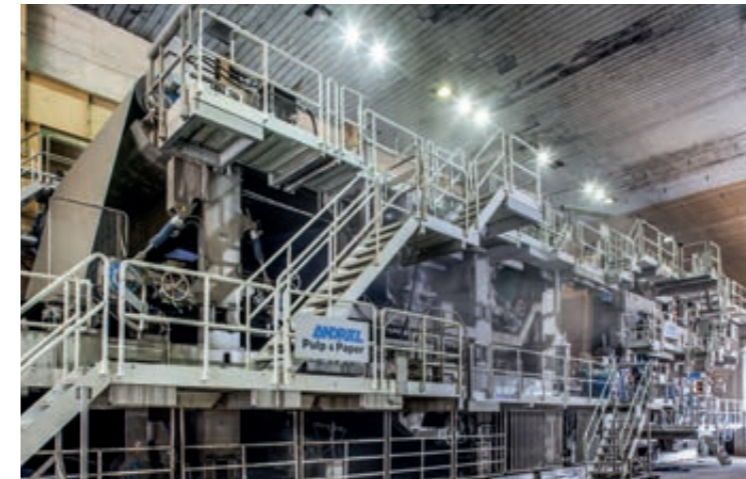
▲ Photo shows part of the new top former in the wire section. The original machine had multi-layer forming on seven vacuum formers.
