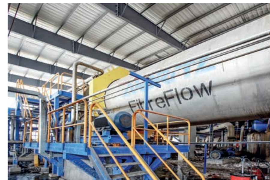
Three of the four layers of the new white-coated board are processed by new ANDRITZ stock preparation systems. Shown here is one of two FibreFlow drum pulpers for processing recycled fiber. ▼
