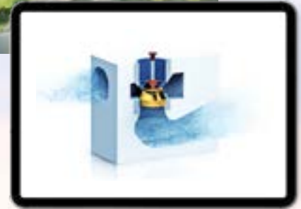
Doan Ha pumping station, two concrete volute pumps
