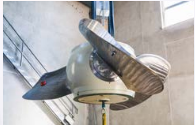
Picture 2: Fish-friendly runner enhancement for the Eddersheim hydropower plant in Germany.
