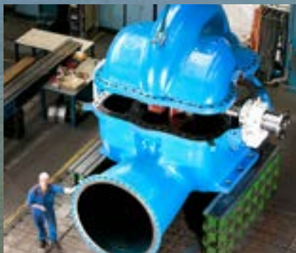
Hui Nan Zhuang, 8 horizontally split double-suction pumps
