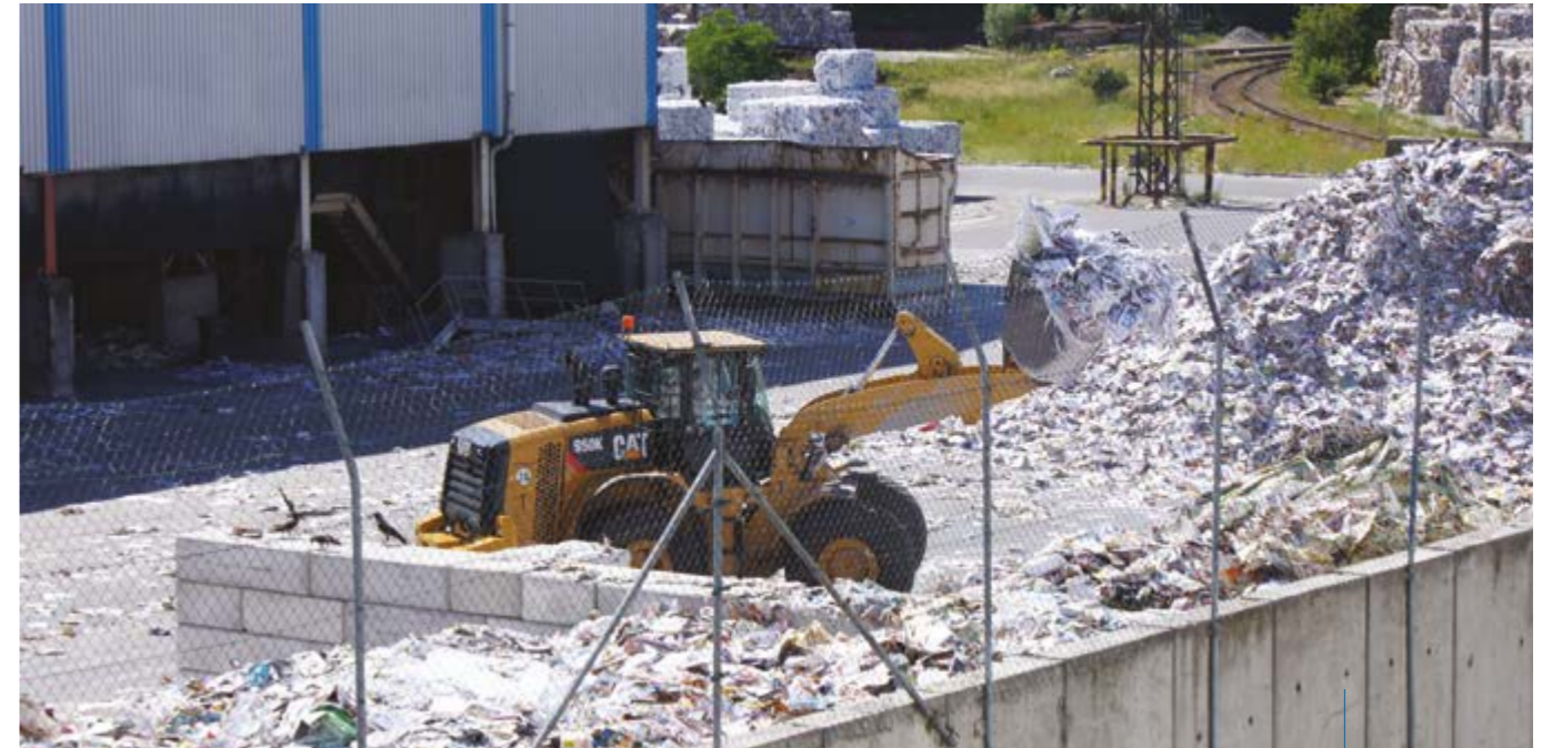
Loose deinking material (illustrated magazines and newsprint) and coated magazines are fed to DIP1.
