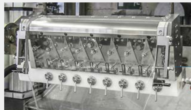
Figure 1. Prototype of new nozzle with sectional volumetric correction of the CD profile.
