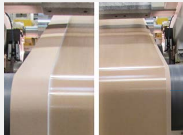
Figure 4. Comparison immediately after coating: with conventional mechanical system (left) and with ANDRITZ edge guide system (right).
