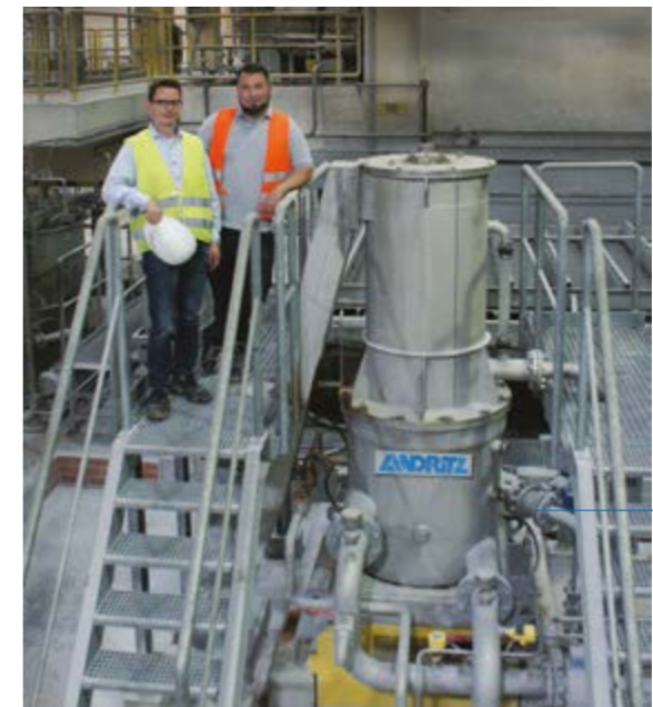
Sebastian Stockfisch, head of deinking and effluent treatment at LEIPA (right), and Markus Mairitsch, ANDRITZ project manager, beside the new ModuScreen T4C tailing screen.
