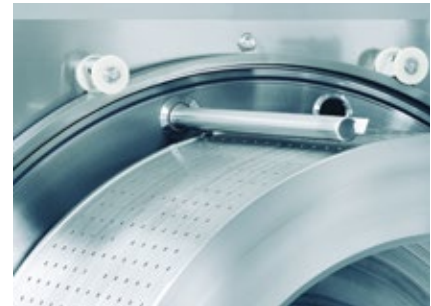
Pneumatic removal of residual heel
