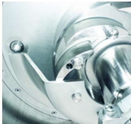
Vane-type feed distributor
